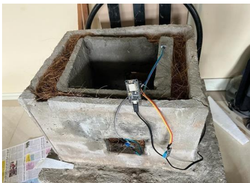
Fig. 3.6: Concrete Cavity Wall Prototype with Insulation
